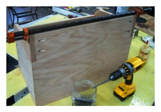
**Step 4: Cut and Attach the Side Supports** - Select the 3/4" Hardwood and the assembled Pieces from Step 3
