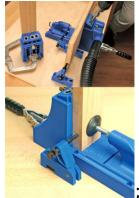
; drill the holes along the interior edges of the Pieces, as shown above
