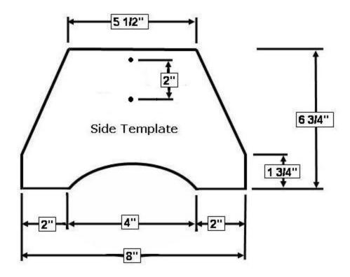
**Step 3: Make A Side Template** - Select a piece of heavy cardboard or thin wood and make a template using the dimensions as shown above.
