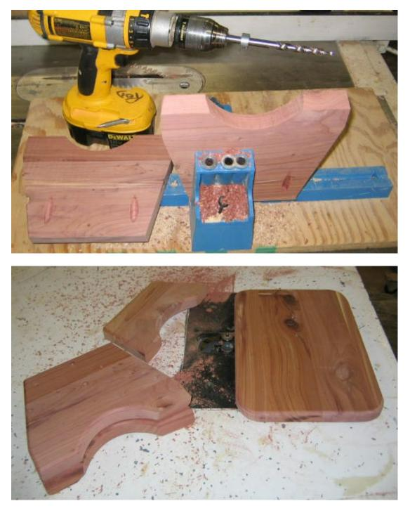
**Step 5: Cut the Sides and Center Support** - Select the Side Template and two, Side pieces; Select the Center Support Template and the Support piece.
