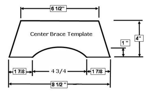
**Step 4: Make A Center Support Template** - Select a piece of heavy cardboard or thin wood and make a template using the dimensions as shown above.
