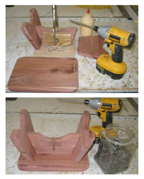
**Step 6: Make an Assembly Jig** - Select some 3/4" plywood and build a 15 degree Assembly Jig as shown above
